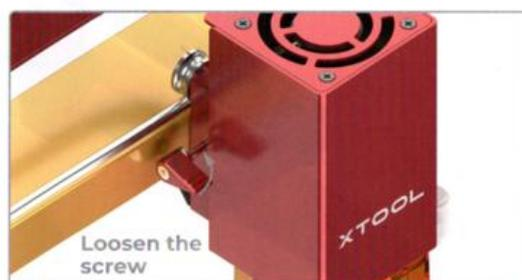
If the handle is blocked, you can tighten or loosen the screw as follows.
